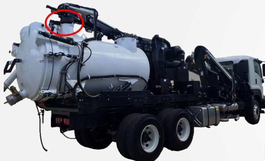
S series is our open housing slewing drive, which is widely applied on engineering machinery. S slewing drive is semi enclosed structure design and is convenient for refueling. S series is suitable for severe conditions and short maintenance application. S series is easy to inspect and maintain. It is an economical and practical choice for clients.
