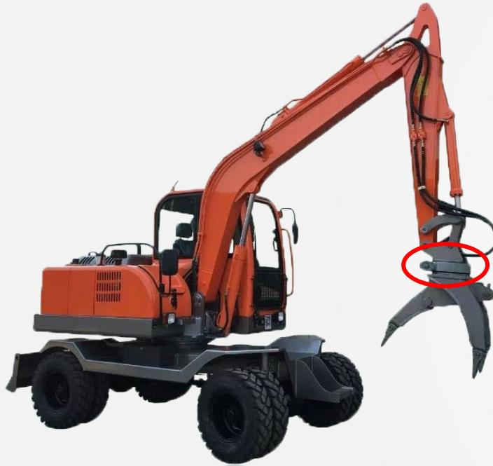
SDL series is the upgraded version of SD series, which has rigorous structure and full sealing. Hourglass worm slewing drive is designed with much tooth contact surface between the worm and gear. The slewing bearing is machined by quenching treatment with stronger hardness, abrasive resistance and longer use life. We use framework oil sealing on SDL series of slewing drives. The sealing is made up of double lip arrangement, high quality steel and NBR. So, SDL slewing drive has higher IP class.
